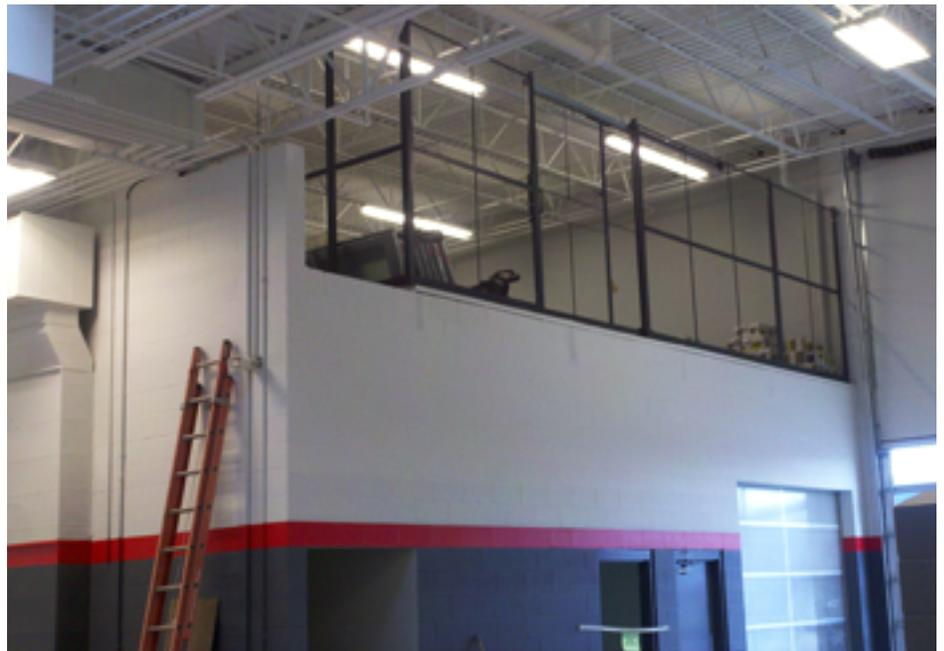
ISS worked with the building architect to ensure the solution for Mini Cooper was satisfactory for all parties involved. As shown in the photos, WireCrafters [wire partitions](#) were used to protect and secure large automotive parts from falling down to the work floor.
